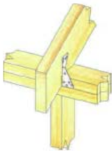
Typical RT3 truss/rafter to plate installation
